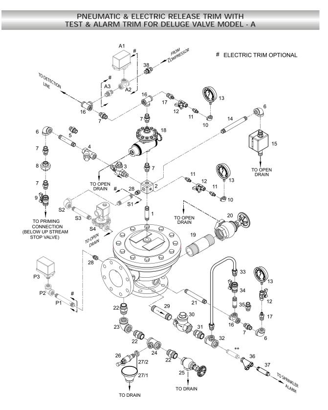
NOTE: WHEN ELECTRIC TRIM IS SUPPLIED THEN SL.NO.28 PLUG NOT REQUIRED.
