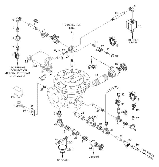
NOTE: WHEN ELECTRIC TRIM IS SUPPLIED THEN SL.NO.28 PLUG NOT REQUIRED.
