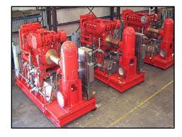
Integral drip-rim base with drain system. Removable 316 SS diesel fuel day tank. Cooling loop with 90-10 copper nickel piping, NiAlBrz body ball valves and regulators. Fiberglass battery boxes with dual Ni-Cad battery banks. Purged NEMA 4X fire pump control panel and engine instrumentation panel. Hydraulic manual secondary engine starting system
